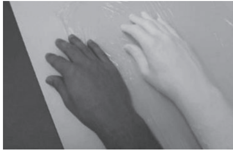
Figure 5.19 Skin-equivalent phantom representing an arm and a hand: (left) human arm used to make a realistic mould and (right) phantom [6]. © 2013 IEEE
