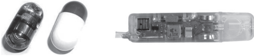
Figure 6.2 Wireless telemetry capsules: (left) BodyCap eCelsius capsules and (right) Bravo pH – image courtesy of Given Imaging Ltd.
