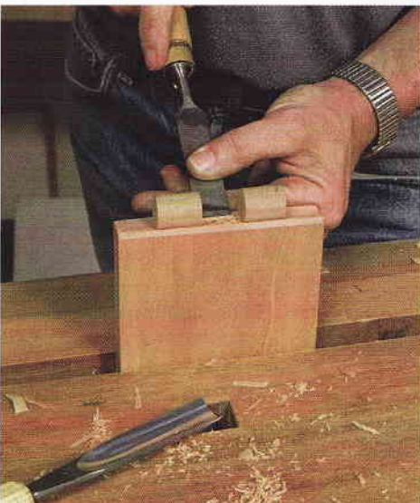
Scoop out the center sockets with a straight chisel. Cove the outside sockets with a gouge of appropriate radius.
