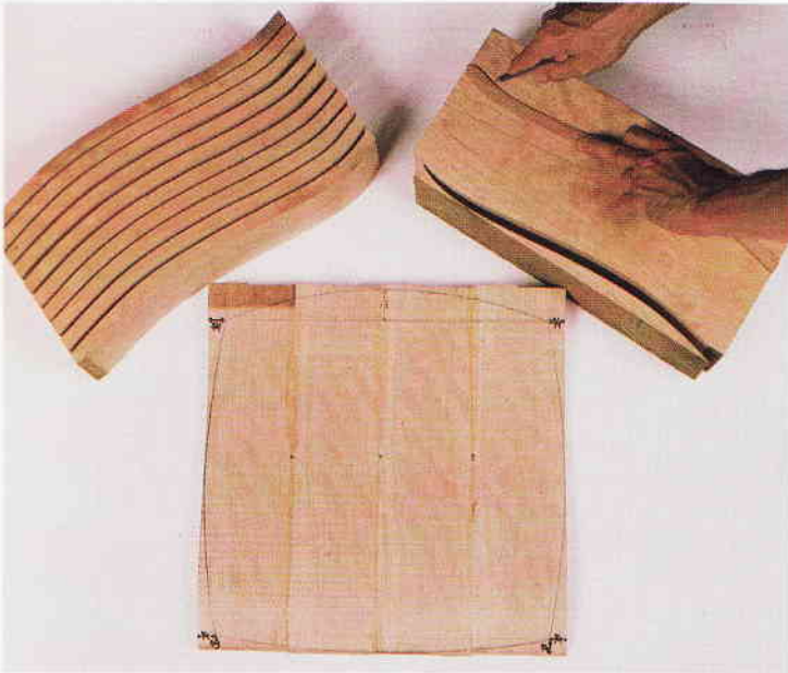
Quartersawn blank from flatsawn stock. Quartersawn lumber is more stable than flatsawn and is easier to grain-match, but it's hard to come by and more expensive. By starting with thicker stock and laying out adjacent seat parts on top of each other across a board's width, the author created quartersawn parts.
