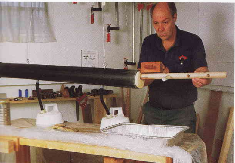
The author's steamer consists of two kettles with built-in electric hot plates that feed steam through dishwasher hose into a length of plastic pipe. Because only the upper end of the back uprights are bent, Oldfield made a wood plug through which he could insert the tapered upper portion of the upright. The short alignment peg in one of the rung holes reminds him of the direction of the bend.
