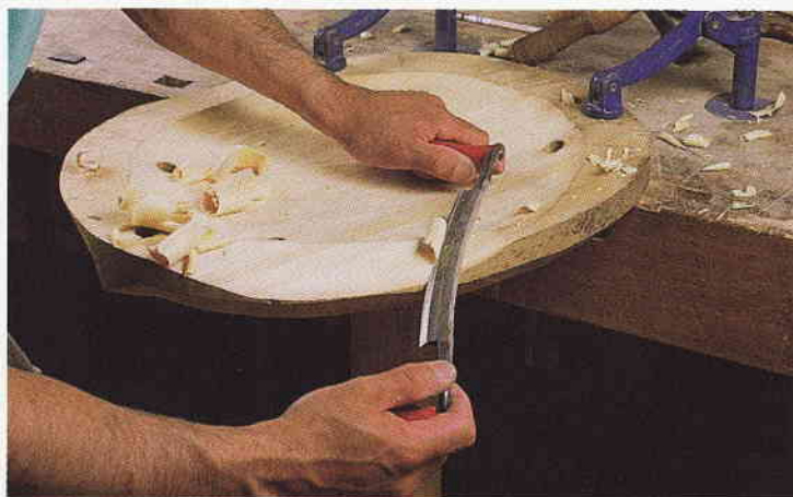
Step 3: Shape convex surfaces with a drawknife.
