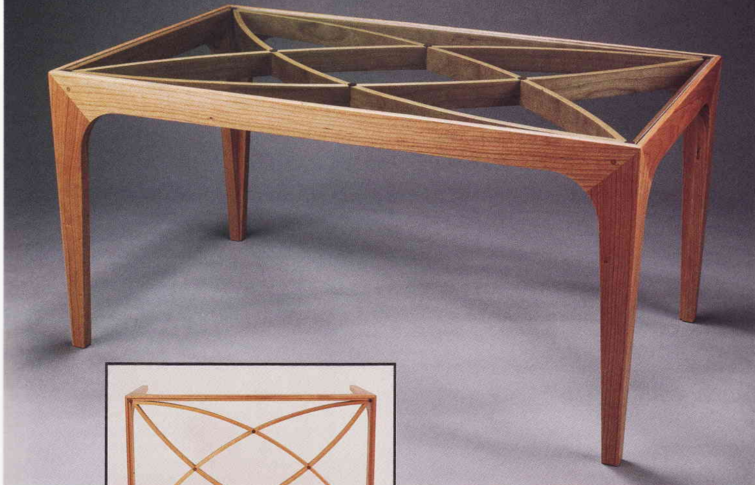
Becksvoort made this glass-top coffee table from 3/4-in.-thick stock rescued from the scrap bin. The legs are mitered together at the corners and also mitered to the aprons, so there is no endgrain showing on the finished table. The inset photo shows the gently curving shapes created by the bent-laminated glass supports.
