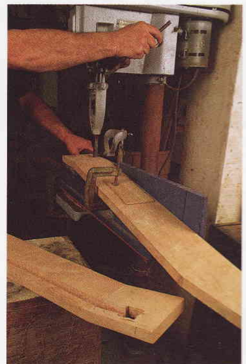
Using a hollow-chisel mortiser attachment on the drill press makes quick work of cutting the through-mortises in the chair's arms to take the leg tenons. The same device also works to cut the groove under the arm to fit on the side rails, as shown on the already-cut arm in the foreground.
