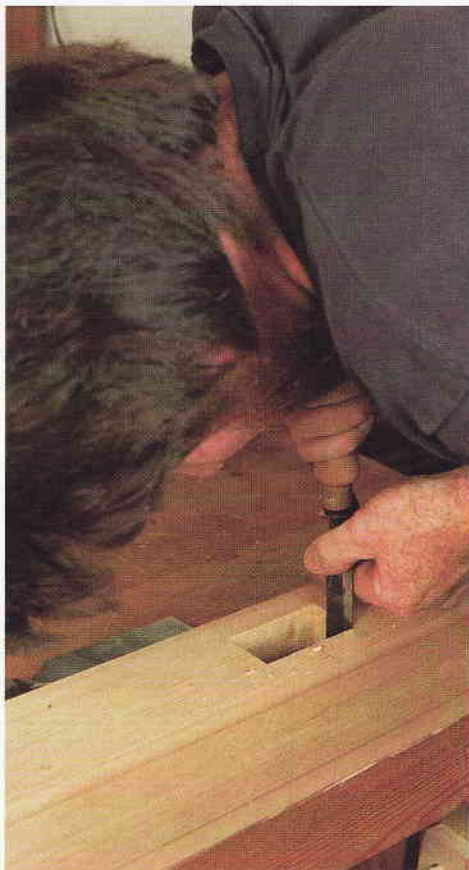
A sharp paring chisel will smooth and square the walls of the mortise (above), ensuring a good, snug fit of an accurately sized tenon in the trestle.
