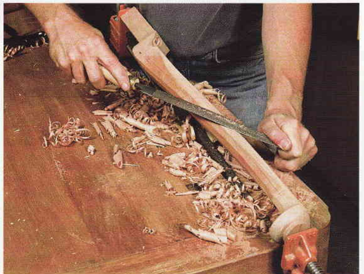
Shape and blend the curves of the cabriole legs with rasps and files. The leg should be round at the ankle and square with rounded corners just below the knee.
