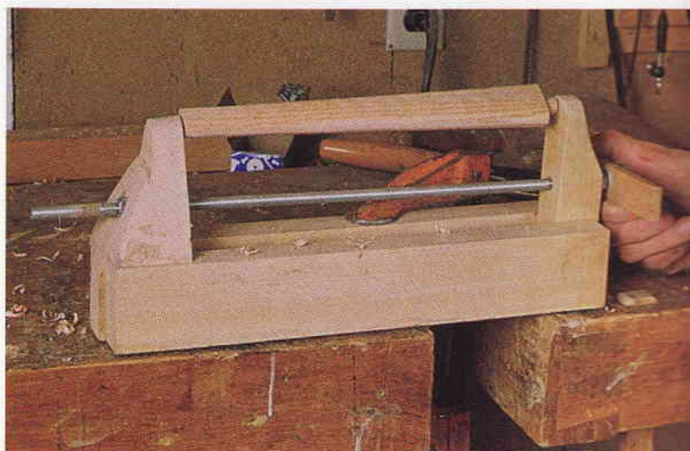
This clamping fixture holds the spokes tightly, yet allows them to be quickly rotated, to speed up the process of handplaning the spokes so that they taper from oval at one end to round at the other.
