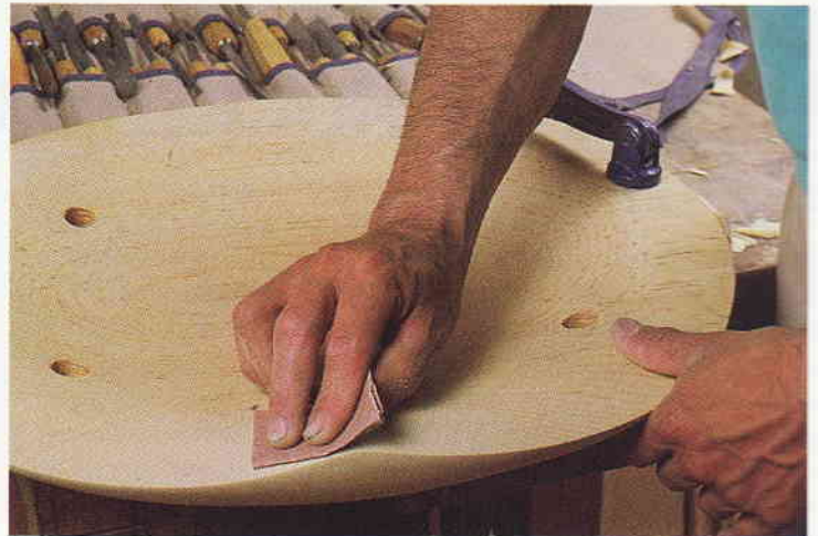
Step 6: Smooth the seat contour with sandpaper.
