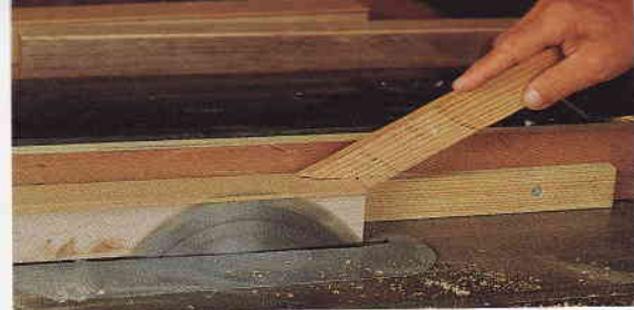
Above: Excess laminate on one side of the walnut leg extends over a 1 \frac{1}{2} -in.-high auxiliary fence as the excess is ripped from the leg's other side. Below: After clamping a leg in the mortise jig, Frid guides the router fence against the jig's side and gauges the mortise's length with the jig's stops.
