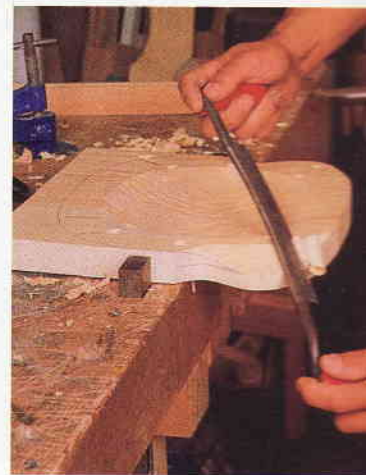
Above: Rodriguez scoops out the saddle with an inshave. Since the tool's long, angled handles prevent him from cutting steeply into the seat, he'll finish around the back edges with a wide gouge. Right: The author carves the front of the seat to a line that is marked on the middle of the edge and that curves around the sharp corner where the top rolls over. Below: Rodriguez steam bends the combs for about 45 minutes in a closed plastic pipe connected to a wallpaper steamer. Then the combs can be wedged against forms on his plywood bending fixture.
