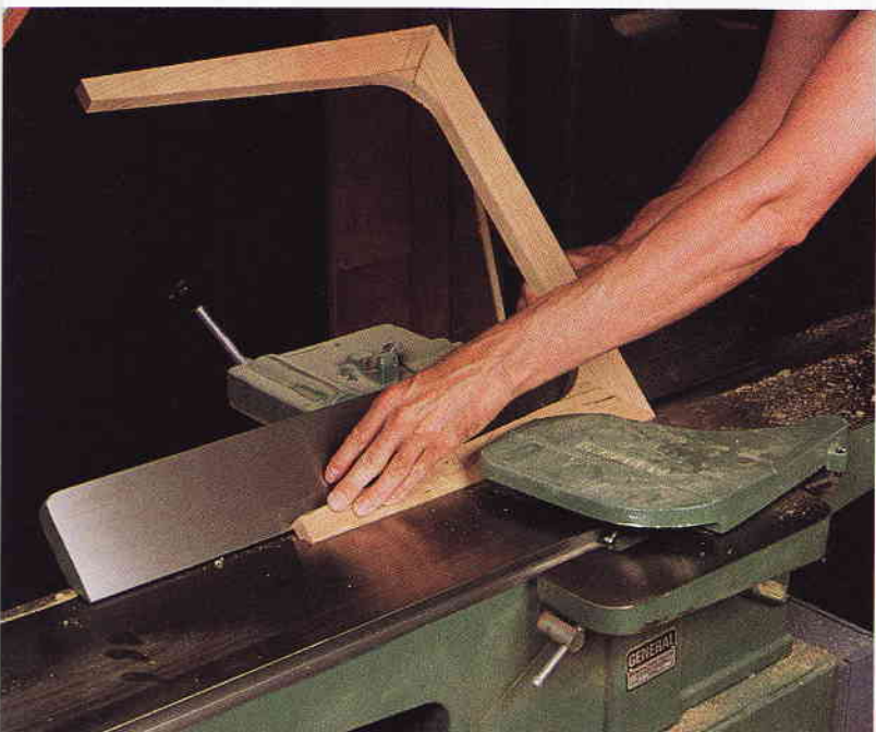
Mitering the edges of the legs on the jointer is easier and provides better results than doing them on the tablesaw.
