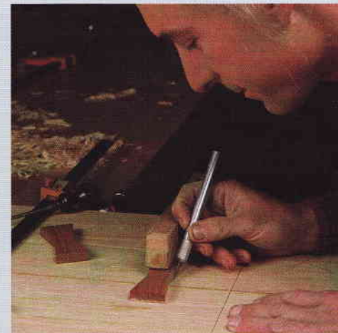
1) Scribe the outline of the key with a knife or an awl.
