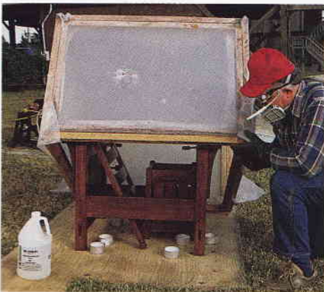
Using 26% ammonia to fume the wood gives distinctive color, but rubber gloves, protective eyewear and breathing apparatus are a must. Cups of ammonia are placed inside the plastic-sheet fuming tent with items to be fumed and left overnight.
