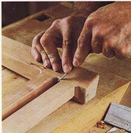
Filing between mortise sockets (above) is one of the final steps to complete the chamfered details before the table frame halves are glued together.
