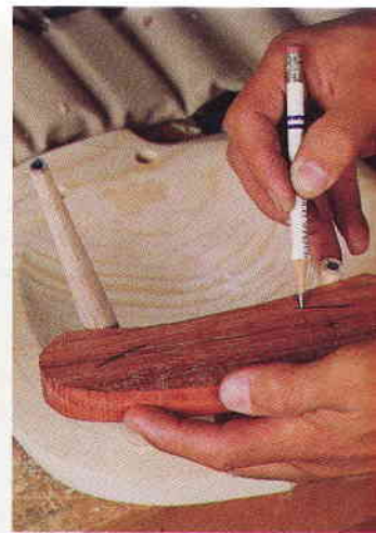
Left: Before drilling the armrest for the back posts and arm posts, the author holds it in position and marks the edge where each post will meet it. Then he sights the direction to point the drill, where each post appears plumb, and marks direction lines on the top of the armrest ( right ).
