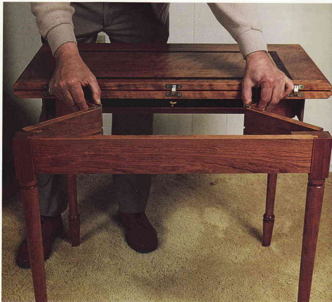
A 200-year-old Dutch table was the model for the author's interpretation, shown above and at right. An ingenious folding-rail system allows the table to do double duty as a simple hall table most of the time and as a game table when the need arises.
