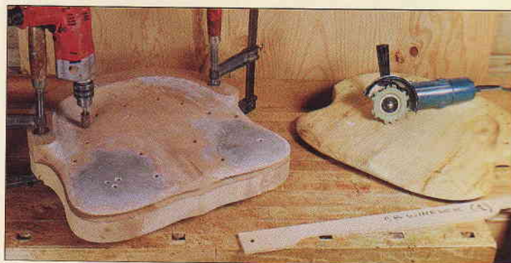
Both Bill Turner and Mac Campbell use depth holes to guide them when roughing out seats. Campbell modified the shape of this pattern (left) several times by adding fiberglass auto-body compound and grinding away wood. As he's carving, he periodically checks the seat's profile with a centerline template.
