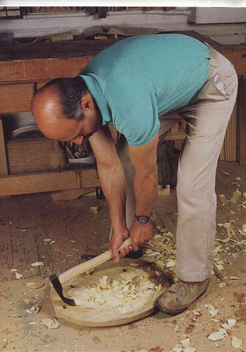
Step 1: Rough the seat hollow with an adze.
