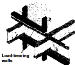
Figure 4-13 BLOCKING PANEL (COURTESY OF BOISE CASCADE CORPORATION)
