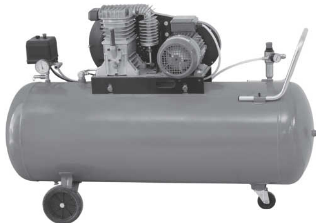
FIGURE 1.20 Air compressor with tank.
