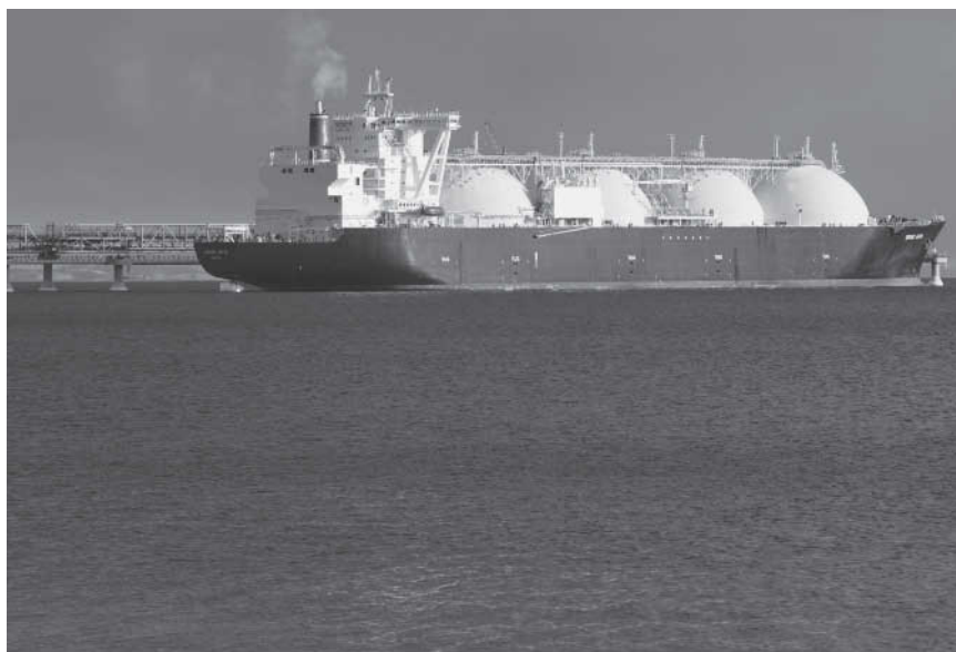
FIGURE 2.24 A tanker to transport liquefied natural gas (LNG), which is mainly methane.
