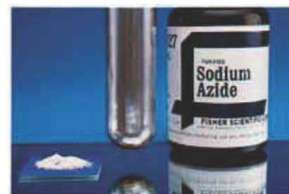
Figure 10.12 When sodium azide, \text{NaN}_3(s) , is heated in a vacuum, it decomposes into nitrogen gas and sodium metal vapor. The sodium metal vapor condenses on the wall of the tube to form a sodium mirror.
