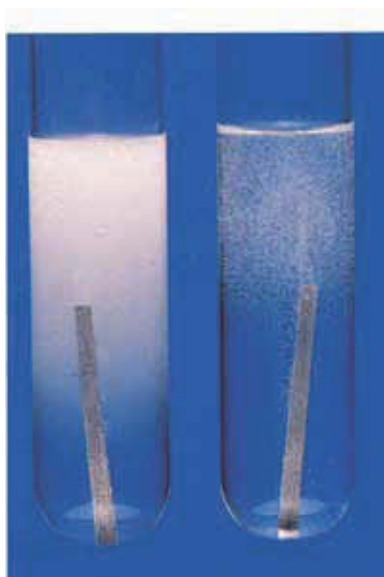
Figure 20.4 The reactions of a strong acid (left) and of a weak acid (right) with magnesium. The strong acid produces a much more vigorous reaction.
