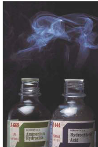
Figure 10.3 Ammonia and hydrogen chloride are colorless gases. They react in a combination reaction to produce the solid white compound ammonium chloride \text{NH}_4\text{Cl}(s) . The white cloud in the picture consists of small ammonium chloride particles formed where the ammonia vapor from one bottle comes into contact with the hydrogen chloride vapor from the other.
