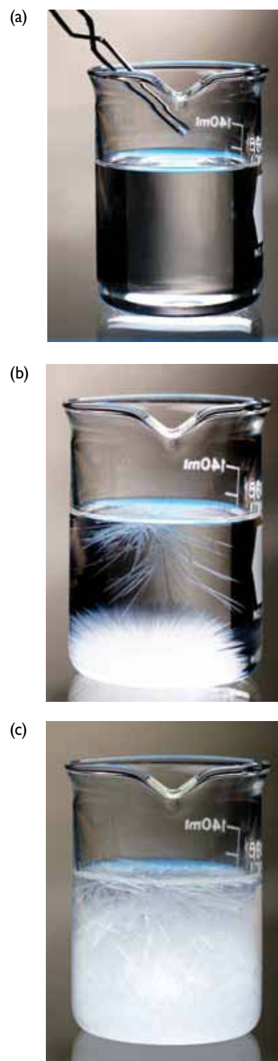
Figure 22.6 A supersaturated solution of sodium acetate, \text{NaCH}_3\text{COO}(aq) . When a single seed crystal of \text{NaCH}_3\text{COO}(s) is added to the solution rapid precipitation occurs.
