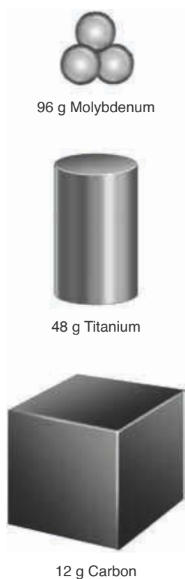
Figure 11.1 12 grams of carbon contains the same number of atoms as 48 grams of titanium and 96 grams of molybdenum.
