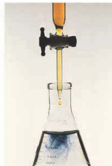
Figure 24.7 The reaction of sodium thiosulfate, \text{Na}_2\text{S}_2\text{O}_3(aq) , in the presence of starch, with \text{I}_2(aq) . Iodine, \text{I}_2(aq) , combines with starch to form a blue starch-iodine complex. When the \text{I}_3^-(aq) ions are reduced by thiosulfate, \text{Na}_2\text{S}_2\text{O}_3(aq) , to iodine, the blue color appears.
