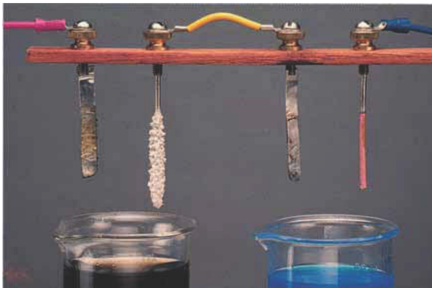
Figure 25.16 Electrodeposition of silver from \text{AgNO}_3(aq) (left), and copper from \text{Cu}(\text{NO}_3)_2(aq) (right). The same quantity of electricity flows through the two solutions because they are placed in series. The number of moles of silver deposited after a given time is twice as great as the number of moles of copper deposited because the reduction of one mole of \text{Ag}^+(aq) requires one mole of electrons, whereas the reduction of one mole of \text{Cu}^{2+}(aq) requires two moles of electrons.
