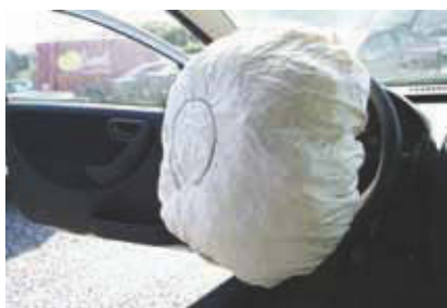
Figure 10.13 An automobile safety air bag undergoes an explosive expansion (driven by nitrogen gas evolution from sodium azide) to provide crash protection for the occupant.
