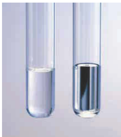
Figure 15.17 A meniscus formed by water ( left ) in a glass tube is concave, whereas the meniscus formed by mercury ( right ) is convex.
