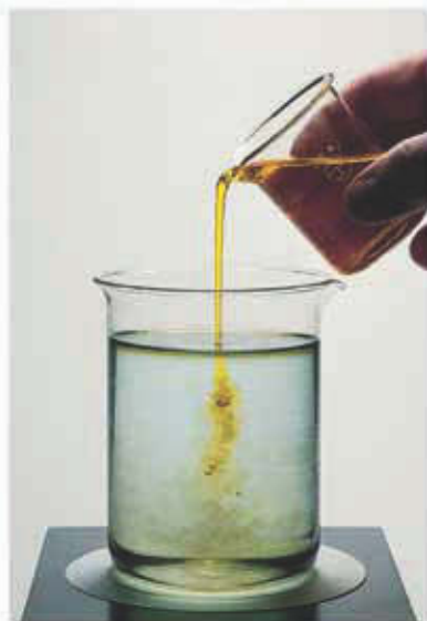
Figure 24.5 Addition of a 0.10-M solution of the oxidizing agent potassium dichromate, \text{K}_2\text{Cr}_2\text{O}_7(aq) (orange solution), to a solution containing 0.10-M iron(II) sulfate, \text{FeSO}_4(aq) (pale green), and 0.10 M \text{H}_2\text{SO}_4(aq) . The iron atom is oxidized from \text{Fe}^{2+}(aq) to \text{Fe}^{3+}(aq) , and the chromium atom is reduced from Cr(VI) in \text{Cr}_2\text{O}_7^{2-}(aq) to Cr(III) in the green \text{Cr}^{3+}(aq) ion.
