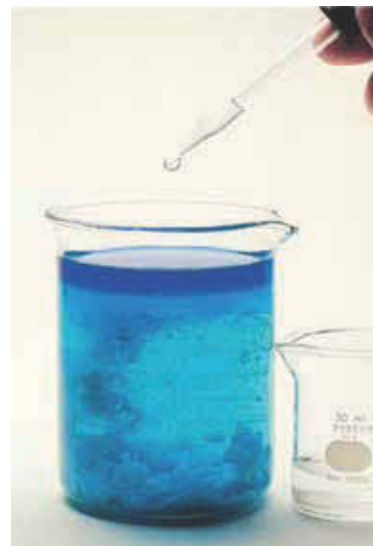
Figure 26.16 A comparison of the color of [\text{Cu}(\text{H}_2\text{O})_6]^{2+}(aq) and [\text{Cu}(\text{NH}_3)_4(\text{H}_2\text{O})_2]^{2+}(aq) (top layer) after the addition of \text{NH}_3(aq) .
