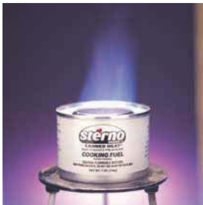
Figure 14.13 A Sterno burner in operation. Sterno is a mixture of ethanol and methanol in a gelling agent, which makes the fuel a solidlike material.
