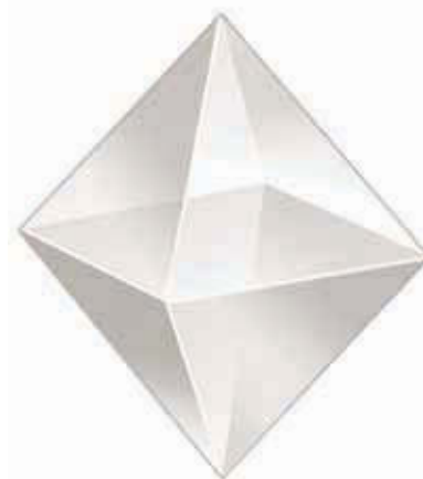
Figure 8.9 A regular octahedron is a symmetric body consisting of six equivalent vertices and eight identical faces that are equilateral triangles.
