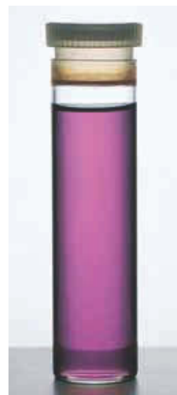
Figure 26.38 An aqueous solution of titanium(III) chloride. The d^1 complex ion [\text{Ti}(\text{H}_2\text{O})_6]^{3+} has a purple color.
