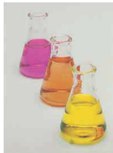
Figure 21.12 Aqueous solutions containing the acid-base indicator methyl red at pH values of 2 (red), 5 (orange), and 10 (yellow).
