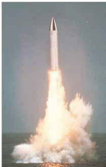
Figure 14.14 Underwater firing of a Polaris A-3 test missile from a nuclear submarine.
