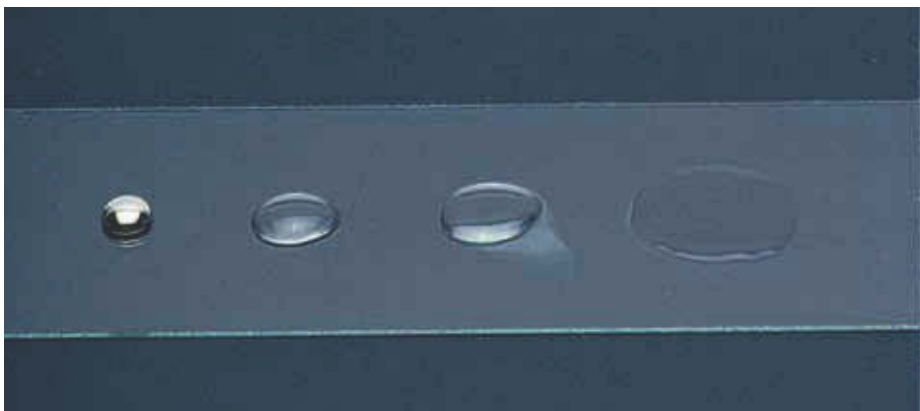
Figure 15.15 Shapes of equal volumes of \text{Hg}(l) , \text{H}_2\text{O}(l) , (\text{CH}_3)_2\text{SO}_3(l) (dimethylsulfoxide), and (\text{CH}_3)_2\text{CO}(l) (acetone), from left to right. Surface tension holds the drops in a spherical shape, and gravity flattens them. The effect of gravity is the same for all the drops; thus, the higher the surface tension, the more nearly spherical is the drop. Surface tension has units of energy per unit area, usually expressed as millijoules per square meter ( \text{mJ}\cdot\text{m}^{-2} ).
