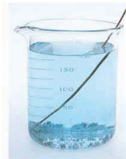
Figure 10.17 (top) A silver nitrate solution, \text{AgNO}_3(aq) , is colorless. (bottom) When a copper wire is inserted, the solution slowly turns blue as a result of the formation of aqueous copper nitrate, \text{Cu}(\text{NO}_3)_2(aq) . Note the silver metal crystals on the bottom of the beaker.
