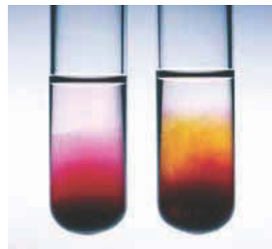
Figure 26.8 An aqueous solution of potassium permanganate, \text{KMnO}_4(\text{aq}) , is a strong oxidizing agent. Freshly prepared \text{KMnO}_4(\text{aq}) is purple (left). As the solution stands, brown \text{MnO}_2(\text{s}) precipitates as a result of the reduction of \text{KMnO}_4(\text{aq}) by \text{H}_2\text{O}(\text{l}) (right).
