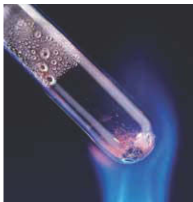
Figure 10.10 When mercury(II) oxide is heated, it decomposes into elemental mercury and oxygen gas. The red compound shown here is mercury(II) oxide. Liquid mercury has condensed on the walls of the test tube and the evolved oxygen gas exits at the tube opening.
