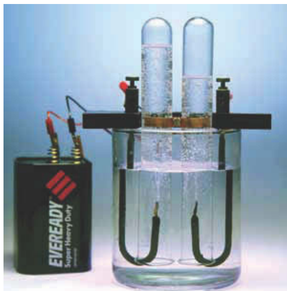
Figure 25.2 Preparation of hydrogen and oxygen by electrolysis of an aqueous solution. Hydrogen gas is liberated at the negative terminal, and oxygen gas is liberated at the positive terminal. As is required by the reaction stoichiometry, the volume of \text{H}_2(g) liberated is twice as great as that of \text{O}_2(g) :
