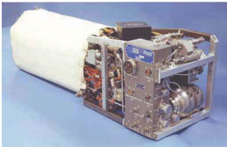
Figure 25.12 The power plant used in the Space Shuttle. Each Space Shuttle is equipped with three hydrogen-oxygen fuel cell power plants. Each power plant is capable of supplying 12 kilowatts at peak output and 7 kilowatts average power to the spacecraft's electrical system.
