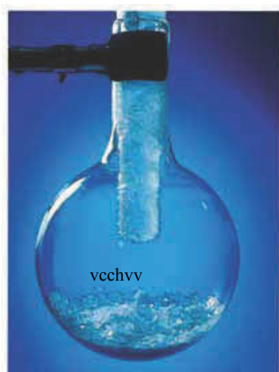
Figure 15.3 Naphthalene, \text{C}_{10}\text{H}_8(s) , is one of a number of substances that readily sublime at room temperature. Here we see crystals of naphthalene condensing directly from vapor to crystals on the surface of a cold tube.
