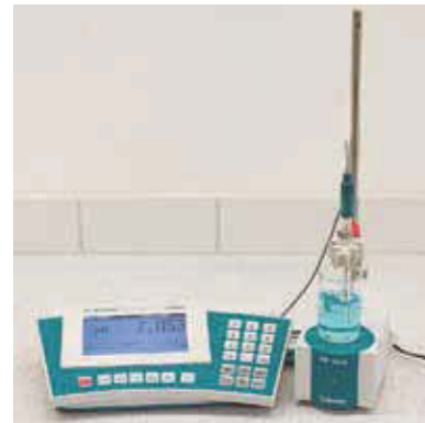
Figure 20.3 A pH meter. A glass electrode sensitive to the concentration of \text{H}_3\text{O}^+(aq) ions is placed in the solution to measure the pH. Such a meter contains a reference solution (which must be changed periodically). Because the concentration of this reference solution changes slowly with time, pH meters must be calibrated periodically using standardized solutions of known pH.
