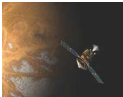
Figure 11.11 The Mars Reconnaissance Orbiter (MRO) was positioned over the surface of Mars using rocket engines powered by a stoichiometric mixture of hydrazine, \text{N}_2\text{H}_4(l) , and dinitrogen tetroxide, \text{N}_2\text{O}_4(l) .
