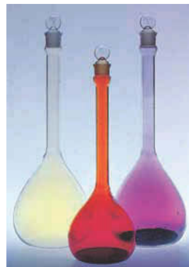
Figure 3.8 Left to right: Chlorine, \text{Cl}_2(g) , bromine, \text{Br}_2(l) , and iodine, \text{I}_2(s) , members of the halogen family. Fluorine is too reactive to be stored in a flask.
