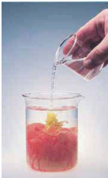
Figure 12.11 A mercury(I) iodide, \text{Hg}_2\text{I}_2(s) , precipitate is produced by the addition of \text{Hg}_2(\text{NO}_3)_2(aq) to \text{KI}(aq) .
