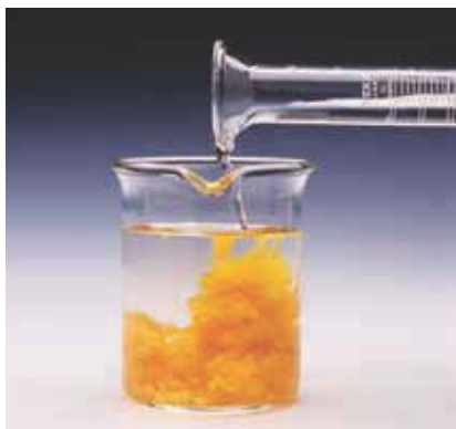
Figure 12.13 When colorless solutions of cadmium(II) nitrate, \text{Cd(NO}_3)_2(aq) , and sodium sulfide, \text{Na}_2\text{S}(aq) , are mixed, a yellow-orange precipitate forms.
