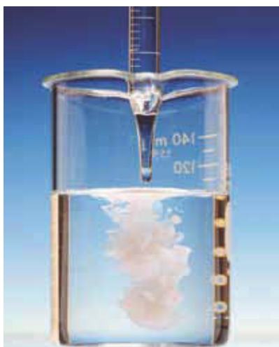
Figure 10.21 The reaction of sodium chloride, \text{NaCl}(aq) , with silver nitrate, \text{AgNO}_3(aq) , yields the white precipitate, silver chloride, \text{AgCl}(s) .
