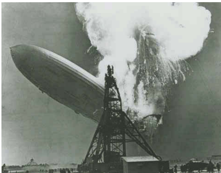
Figure 3.2 The explosion of the hydrogen gas-filled German dirigible Hindenburg during landing at Lakehurst, New Jersey.
