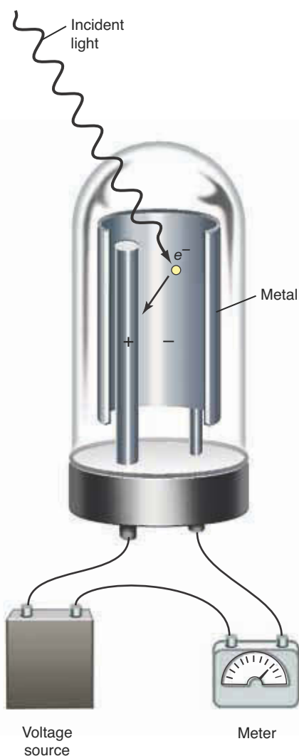
Figure 4.17 An apparatus for studying the photoelectric effect. Light of a certain frequency falls on a clean metal surface, ejecting electrons that are attracted toward the positive electrode. The number of electrons ejected is registered by a detecting meter.
