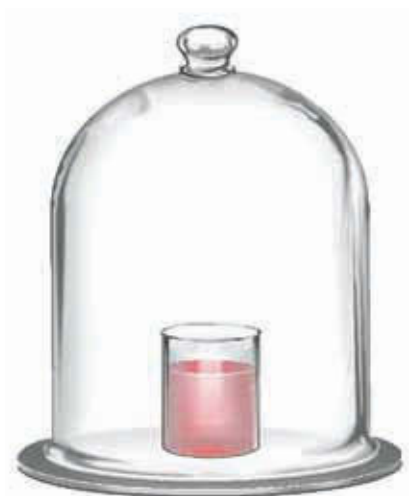
Figure 15.18 When a liquid is placed in a closed container that has been evacuated, the pressure of the vapor above the liquid eventually reaches a constant value that depends upon the particular liquid and the temperature.
