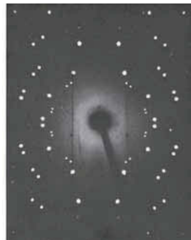
Figure 15.26 The X-ray diffraction pattern produced by a crystal of sodium chloride. The symmetry and spacing of the dots carry detailed information regarding the arrangement of atoms in the crystals.
