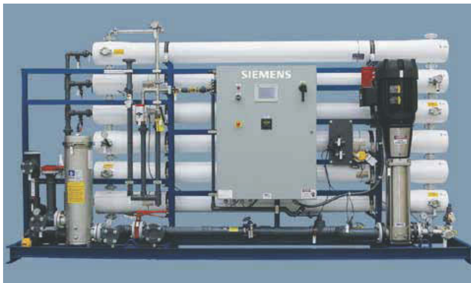
Figure 16.15 A commercial reverse osmosis unit. Suspended solids, including bacteria, are blocked by mechanical exclusion, and dissolved salts are removed using semipermeable membranes (Figure 16.14). The unit shown reduces the salt concentration to less than 5% of the initial concentration.
