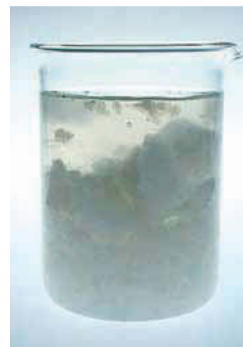
Figure 22.7 Aluminum hydroxide, \text{Al}(\text{OH})_3(s) , occurs as a white, flocculent precipitate that is used to clarify water.
