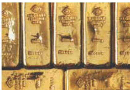
Figure I.16 Gold ingots weighing one kilogram. Each ingot is stamped with its weight, purity, and reference number.
