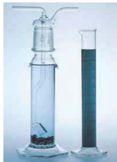
Figure 26.7 Left, a chromous bubbler, which is used to remove traces of oxygen from unreactive gases such as nitrogen or argon. The blue color of the solution is due to \text{Cr}^{2+}(\text{aq}) , and the solid at the bottom of the tube is a zinc amalgam, \text{Zn}(\text{Hg})(\text{s}) . The gas to be deoxygenated enters the bubbler at the left inlet tube, bubbles up through the solution of \text{Cr}^{2+}(\text{aq}) , and exits from the right tube. A glass membrane at the bottom of the inlet tube breaks up the entering gas stream into small bubbles. Right, the green solution in the graduated cylinder is \text{Cr}_2(\text{NO}_3)_3(\text{aq}) , which is used to prepare the chromous bubbler. The green \text{Cr}^{3+}(\text{aq}) is reduced to the blue \text{Cr}^{2+}(\text{aq}) by the zinc amalgam in the bubbler.
