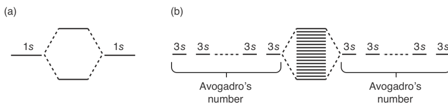
Figure 15.35 (a) When two hydrogen atoms are brought together, their 1s orbitals combine to form a bonding and an antibonding molecular orbital. (b) When Avogadro's number of sodium atoms are brought together to form a sodium crystal, the 3s orbitals (the valence orbitals) of the sodium atoms combine to form Avogadro's number of molecular orbitals that are delocalized over the entire crystal lattice. The energies of these orbitals are so close together that they form essentially a continuum of energy levels, as illustrated schematically here.
