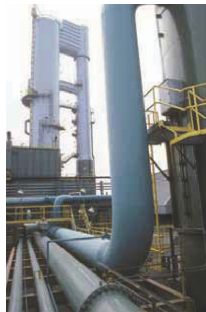
Figure 19.13 An ammonia plant. This plant produces 750 tons of ammonia per day from hydrogen and nitrogen. The nitrogen comes from the air and the hydrogen is obtained from the reaction between methane and steam. Ammonia is used in the production of fertilizers, explosives, polymers, and household cleansers.
