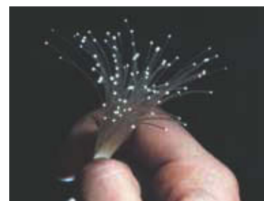
Figure 15.34 Fiber optics. Light is transmitted through thin strands of silica glass that form an optical-waveguide fiber bundle that acts as an optical pathway for the light.
