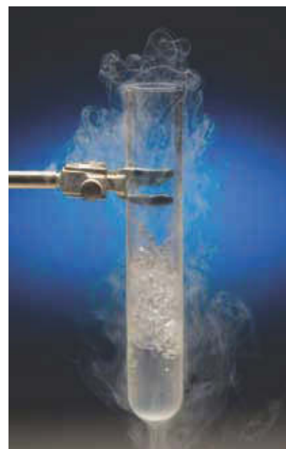
Figure 23.14 Liquid nitrogen has a normal boiling point of 77 K. This photograph shows the liquid boiling at atmospheric pressure. The heat energy necessary to boil the liquid comes from the surroundings at 20^\circ\text{C} . Because the boiling point is so low, no other heat source (such as a flame) is needed to boil the liquid.
