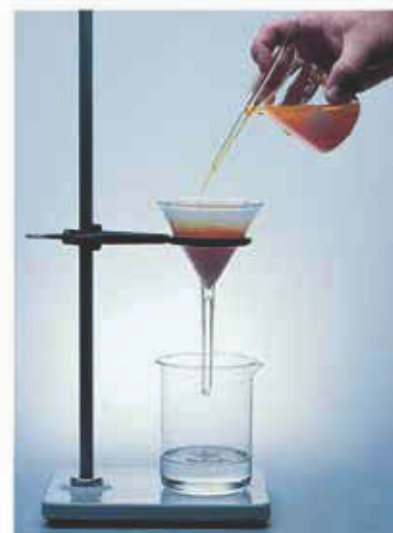
Figure 2.8 Filtration can be used to separate a liquid from a solid. The liquid passes through filter paper, but the solid particles are too large to do so. Filter paper is available in a wide range of pore sizes, down to pores small enough ( 2.5 \times 10^{-8} \text{ m} ) to remove bacteria (the smallest bacteria are about 1 \times 10^{-7} \text{ m} in diameter). Micropore filters can be used in place of pasteurization to produce bacteria-free liquids such as canned draft beer and bottled water.
