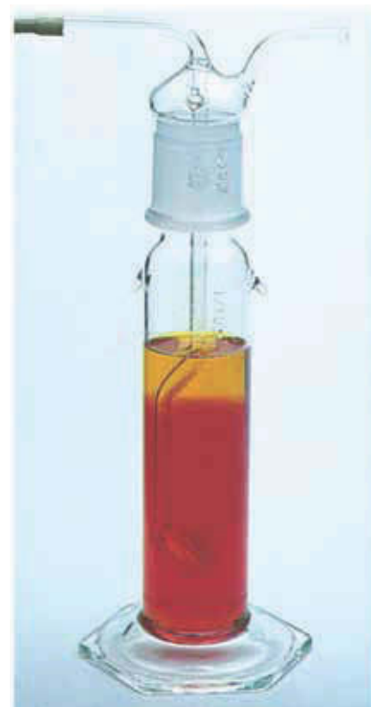
Figure 10.19 When chlorine gas, Cl_2(g) , is bubbled into a colorless aqueous sodium bromide, NaBr(aq) , solution, the chlorine replaces the bromide ions to form sodium chloride, NaCl(aq) , and a reddish-brown solution of bromine in water, Br_2(aq) .
