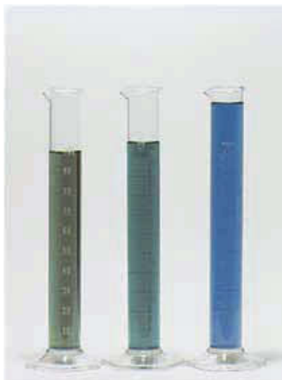
Figure 21.1 The left cylinder contains 100 mL of a sodium acetate and acetic acid buffer solution with bromocresol green indicator that indicates that the pH of the solution is about 5 (see Figure 21.7). The middle cylinder contains 100 mL of the \text{CH}_3\text{COO}^-(aq) – \text{CH}_3\text{COOH}(aq) buffer solution plus 7.0 mL of 0.10 M \text{NaOH}(aq) . The fact that the solution remains green indicates that the pH of the solution is still about 5. The right cylinder contains 100.0 mL of the \text{CH}_3\text{COO}^-(aq) – \text{CH}_3\text{COOH}(aq) buffer solution plus 25.0 mL of 0.10 M \text{NaOH}(aq) . The change in the indicator color from green to blue shows that the pH has increased significantly and that the buffer has been overwhelmed by the addition of a large amount \text{NaOH}(aq) .
