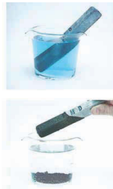
Figure 10.18 (top) A zinc rod is placed in a copper nitrate (blue) solution. (bottom) Zinc has replaced the copper to form a colorless zinc nitrate solution \text{Zn}(\text{NO}_3)_2(aq) . Elemental copper has coated the rod and has fallen to the bottom of the flask.
