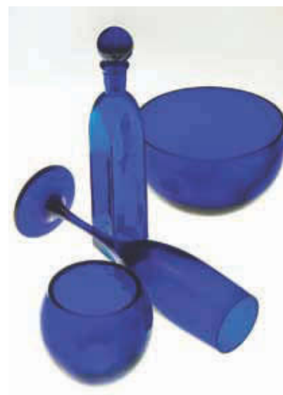
Figure 26.12 Cobalt glass. The characteristic blue color is due to the presence of small amounts of \text{CoO}(s) .
