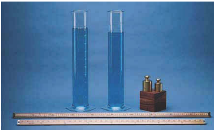
Figure 1.6 Comparison of a meter stick with a yardstick (the meter stick is about 10% longer than the yardstick); a liter with a quart (the volume of a liter is about 6% larger than the volume of a quart); and a kilogram with a pound (the mass of a kilogram is about 2.2 times larger than the mass of a pound).
