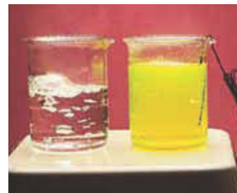
Figure 16.5 Pure water open to the atmosphere boils at 100^\circ\text{C} , whereas a 50-50 mixture by volume of water and automobile antifreeze (ethylene glycol) boils at about 109^\circ\text{C} . The pure water and the antifreeze mixture in this photo are at the same temperature ( 100^\circ\text{C} ), but only the pure water is boiling.
