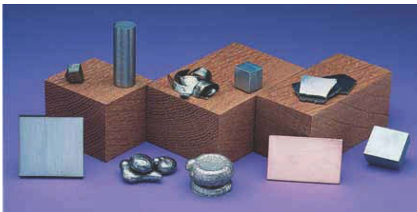
Figure 3.18 The first-row transition series metals. Top row (left to right): Sc, Ti, V, Cr, and Mn. Bottom row: Fe, Co, Ni, Cu, and Zn.
