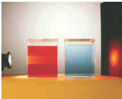
Figure 15.44 An illustration of the Tyndall effect. A colloidal dispersion (red) scatters a beam of light, while a true solution (blue) does not.
