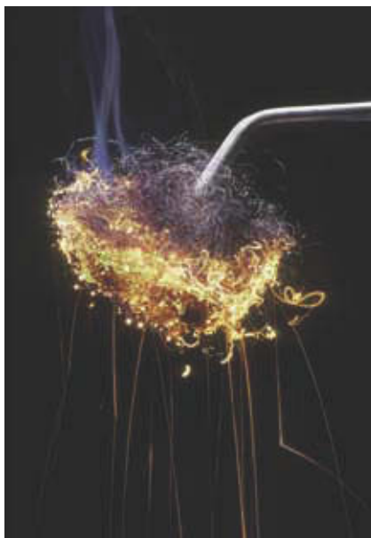
Figure 10.2 Although steel wool does not burn in air, it burns vigorously in pure oxygen.
