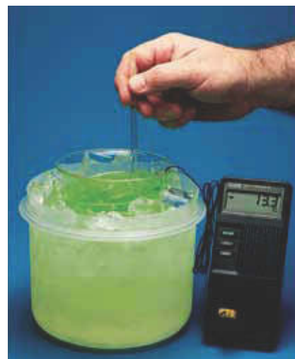
Figure 16.8 A 30% by volume ethylene glycol (automobile antifreeze) and water mixture at -13.3^\circ\text{C} . Note that the mixture remains as a liquid at -13.3^\circ\text{C} , whereas pure water would be frozen solid.
