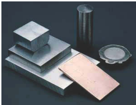
Figure 2.2 Common metals. Clockwise starting with the cylinder at top center are titanium, nickel, copper, aluminum, iron, and zinc.
