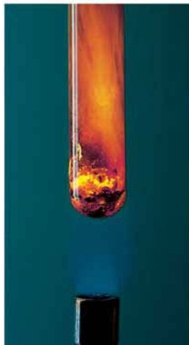
Figure 10.25 The alkali metal sodium reacts with the nonmetal sulfur to produce sodium sulfide.
