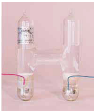
Figure 25.9 A Weston standard cell. The photograph shows the cell in the reverse of the conventional orientation, that is
