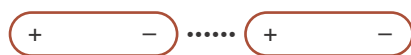
Figure 15.4 Although polar molecules are electrically neutral overall, they attract one another by a dipole-dipole force. The molecules orient themselves as shown because the positive end of one attracts the negative end of another. The dipoles are said to be oriented head-to-tail.
