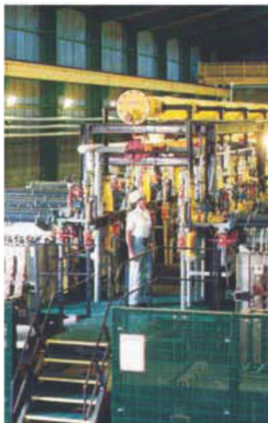
Figure 25.17 A chlor-alkali plant in which chlorine gas and an aqueous solution of sodium hydroxide are obtained by electrolysis from an aqueous solution of sodium chloride.
