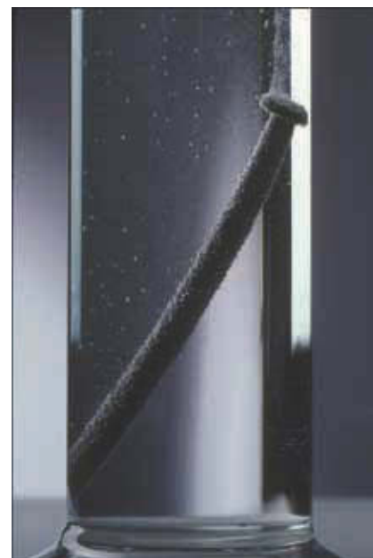
Figure 10.16 The reaction between iron metal and a dilute aqueous solution of sulfuric acid. The bubbles generated at the surface of the iron nail are hydrogen gas. The iron replaces the hydrogen atoms in \text{H}_2\text{SO}_4(aq) and thereby enters the solution as \text{Fe}^{2+}(aq) .
