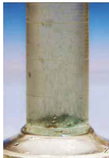
Figure 12.10 Drano® consists of a mixture of pieces of aluminum and \text{NaOH}(s) . When Drano® is added to water, the aluminum reacts with the \text{NaOH}(aq) to produce hydrogen gas.
