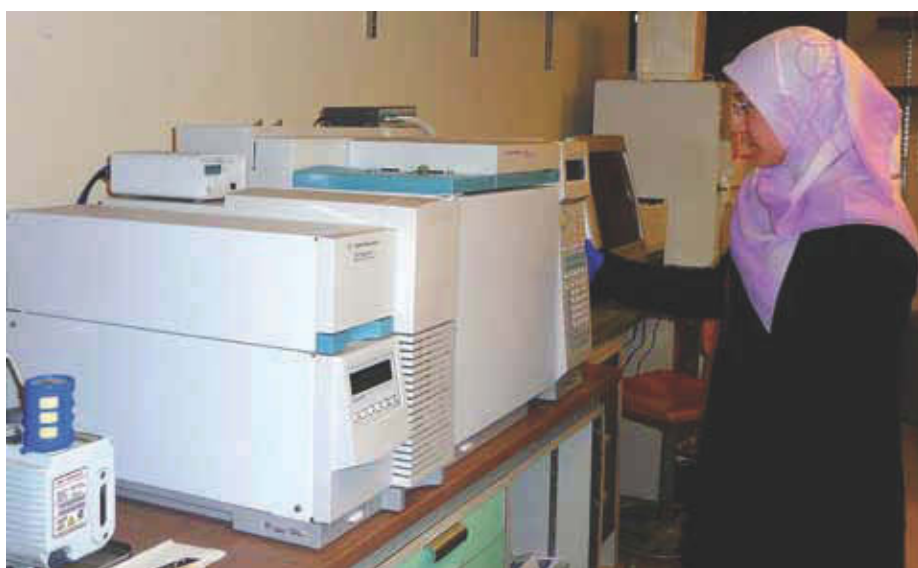
Figure 2.22 A mass spectrometer like the one shown here can be used to separate the isotopes of an element. In addition to determining the mass of isotopes, mass spectrometers are also a powerful tool for chemical analysis. The mass spectrometer shown here is used by students to check for traces of cocaine on U.S. currency.
