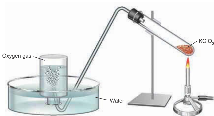
Figure 11.6 A typical experimental setup for the production of small amounts of oxygen by gently heating potassium chlorate, \text{KClO}_3(s) . Because it is only slightly soluble in water, the oxygen is collected by the displacement of water from an inverted bottle.
