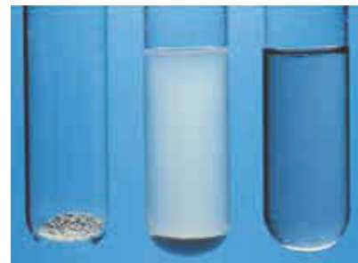
Figure 22.3 Silver bromate is only slightly soluble in water at 25^\circ\text{C} . If \text{NH}_3(aq) is added to a saturated solution of \text{AgBrO}_3(aq) , the solubility of \text{AgBrO}_3(s) is increased as a result of the formation of [\text{Ag}(\text{NH}_3)_2]^+(aq) complex ions. ( left ) Test tube with 1.0 \text{ gram of AgBrO}_3(s) . ( center ) Test tube with 1.0 \text{ gram of AgBrO}_3(s) and 20 \text{ mL of water} . ( right ) Test tube with 1.0 \text{ gram of AgBrO}_3(s) and 20 \text{ mL of } 6 \text{ M NH}_3(aq) .
