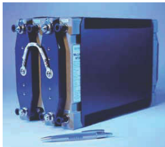
Figure 25.13 This fuel cell stack produced by Ballard Power Systems in British Columbia can deliver up to 1030 watts of electrical power from hydrogen gas. About 15 of these stacks can generate enough energy to power a medium-sized four-passenger electric car with only pure water as a waste product.
