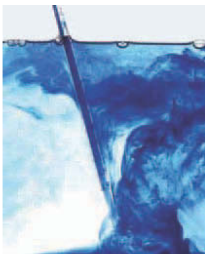
Figure 23.16 The dispersal of ink throughout the entire volume of water is an example of a spontaneous process.
