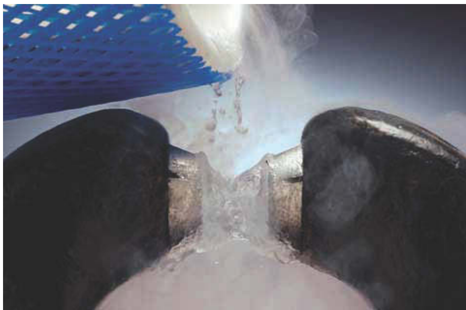
Figure 9.12 Liquid oxygen is attracted to the magnetic field between the poles of a magnet because oxygen is paramagnetic. The attraction of paramagnetic materials to a magnetic field is much weaker than that of ferromagnetic materials (such as iron), and so a strong magnet is used to illustrate this effect.
