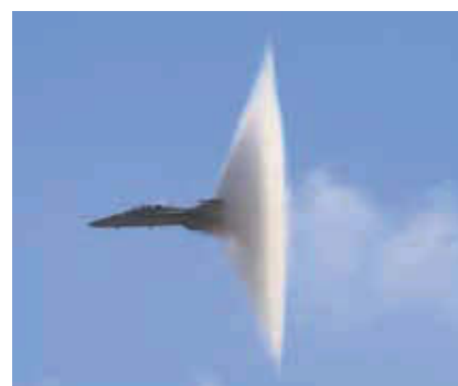
Figure 13.27 When an aircraft first breaks the sound barrier, the sudden change in pressure can condense the water vapor in the atmosphere, forming a vapor cloud in the wake of the plane.
