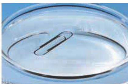
Figure 15.11 A metal paper clip floats on water because of the distribution of its mass and the high surface tension of the water. The surface of water is like an elastic skin that resists penetration.
