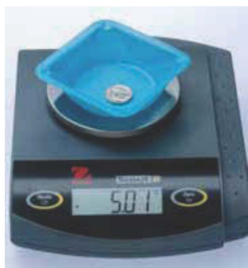
Figure 1.9 ( top ) An automatic analytical balance, ( middle ) a laboratory beam balance, and ( bottom ) an electronic mass scale; are all used to determine mass. The beam balance requires the placement of standard masses on one of the pans to achieve a mass balance.
