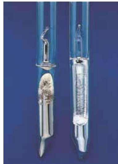
Figure 3.11 Cesium (golden color) and rubidium (silver color) are stored in vacuum-sealed ampoules to prevent their reacting with air.
