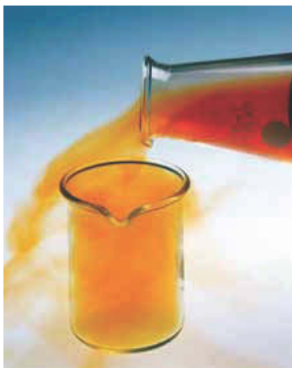
Figure 13.18 Like liquids, gases have flow properties and can be poured from one container to another if they are denser than air. This photo shows \text{NO}_2(\text{g}) being poured.
