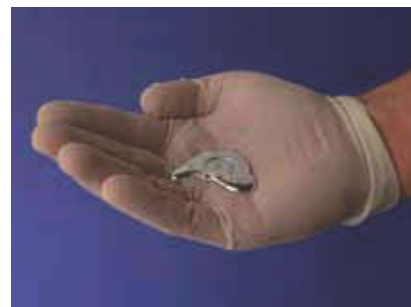
Figure 3.13 Gallium metal has a melting point of 30°C and therefore melts when held in the hand (human body temperature is about 37°C).
