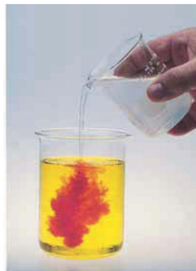
Figure 12.12 A silver chromate, \text{Ag}_2\text{CrO}_4(s) , precipitate is produced by the addition of \text{AgNO}_3(aq) to \text{Na}_2\text{CrO}_4(aq) .
