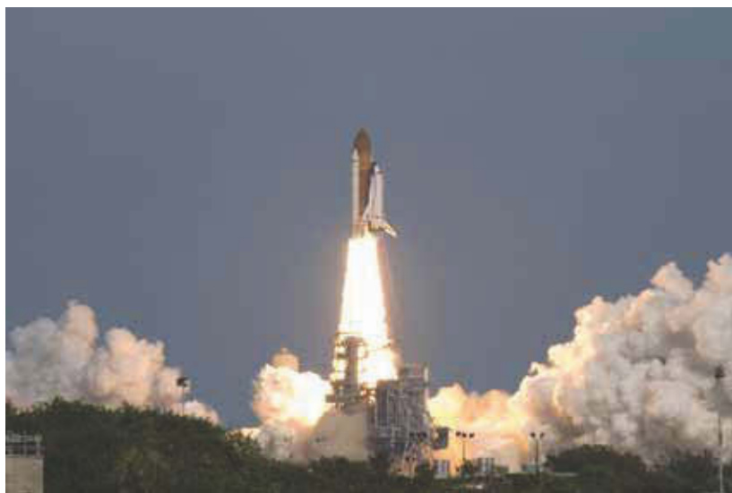
Figure 14.1 Blastoff of a space shuttle. The energy released by the three main engines is equivalent to the output of 23 Hoover Dams. The two solid rocket boosters on the sides of the main fuel tank consume 5 metric tons of fuel per second and generate a combined thrust equivalent to 44 million horsepower, which is equivalent to the horsepower of 15 000 six-axle diesel locomotives or 400 000 subcompact cars.
