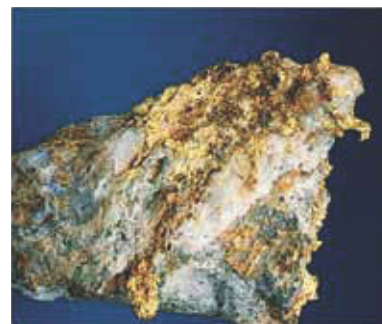
Figure 26.17 Gold often occurs in the free state in nature. Here we see native gold on a quartz crystal.
