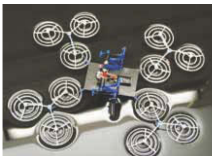
Figure 15.12 (top) Some insects like this water strider use surface tension to walk on water. (bottom) Researchers at Carnegie Mellon University are working to develop a microrobot that uses surface tension to walk on water.
