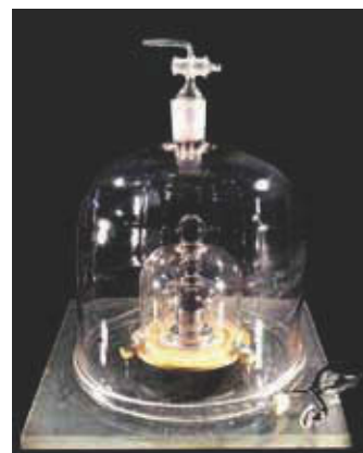
Figure B.1 The U.S. National Prototype Kilogram is currently the primary standard for measuring mass in the United States. It is periodically recertified against the primary international standard Kilogram held at the Bureau International des Poids et Mesures in Sèvres, France (pictured here).
