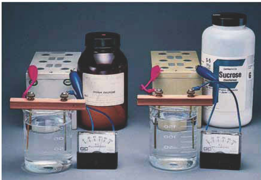
Figure 6.2 Comparison of the currents (as measured using ammeters) through equal concentrations of sodium chloride, \text{NaCl}(aq) , and sucrose, \text{C}_{12}\text{H}_{22}\text{O}_{11}(aq) . The solution of the strong electrolyte, \text{NaCl}(aq) , is a much better conductor of electricity than the solution of the nonelectrolyte, \text{C}_{12}\text{H}_{22}\text{O}_{11}(aq) .
