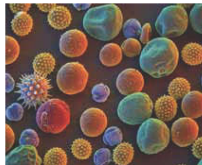
Figure 4.21 An electron micrograph of pollen particles collected by filtering a pollen-laden air sample. The pollen grains range in size from about 15 \mu\text{m} to 40 \mu\text{m} .
