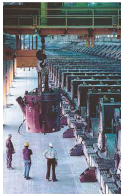
Figure 25.22 The Hall-Héroult process on an industrial scale. Shown here is an Alcoa potline (198 pots) at the Massena, New York, plant.
