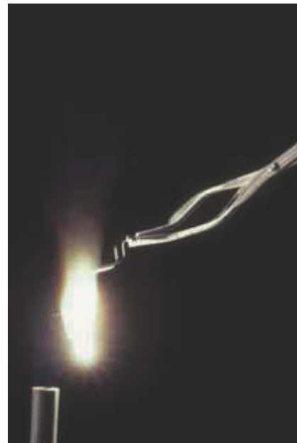
Figure 3.7 Magnesium ribbon burns rapidly in oxygen to form magnesium oxide, a white solid. Magnesium is used in flares, fuses, and pyrotechnics.
