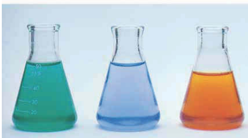
Figure 26.23 Aqueous solutions of Ni(II) complex ions: [\text{Ni}(\text{H}_2\text{O})_6]^{2+}(aq) (green), [\text{Ni}(\text{NH}_3)_6]^{2+}(aq) (blue-violet), and [\text{Ni}(\text{CN})_4]^{2-}(aq) (orange-yellow).
