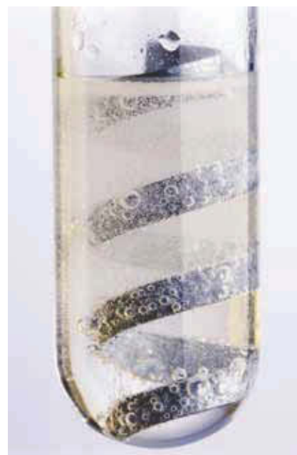
Figure 12.9 Zinc metal reacts with an aqueous solution of hydrochloric acid. The bubbles are hydrogen gas escaping from the solution.
