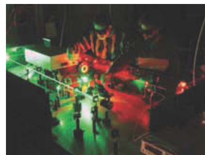
Figure 4.11 Lasers are used to study a wide variety of chemical reactions, ranging from the simplest (e.g., \text{D} + \text{H}_2 \rightarrow \text{HD} + \text{H} ) to the most complex (e.g., combustion reactions). Lasers provide incredible details regarding the energy transfer processes involved in chemical reactions. Lasers are also used in the bar readers at supermarkets, in CD and DVD players, in surgery, in the manufacture of precision mechanical parts, and in many other applications. The development of modern quantum theory led to the invention of the laser.
