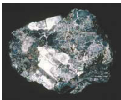
Figure 2.12 Metal sulfides are valuable ores of metals. Shown here is galena, \text{PbS}(s) , the principal ore of lead.
