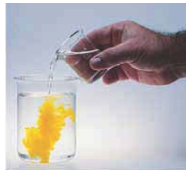
Figure 10.22 When colorless aqueous solutions of cadmium nitrate, \text{Cd}(\text{NO}_3)_2(aq) , and sodium sulfide, \text{Na}_2\text{S}(aq) , are mixed, an orange precipitate of cadmium sulfide, \text{CdS}(s) , forms immediately.
