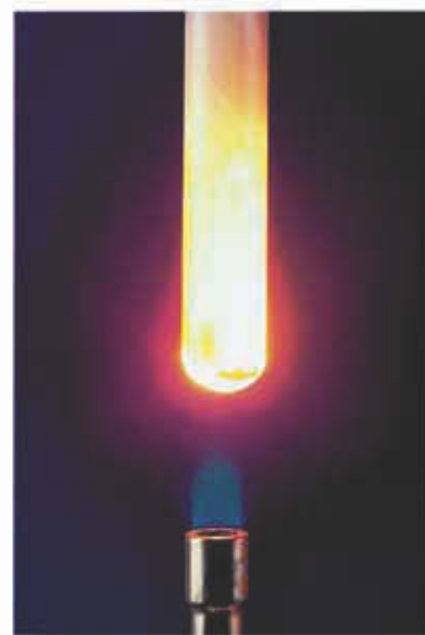
Figure 2.11 The reaction between the elements calcium and sulfur yields calcium sulfide, \text{CaS}(s) . The calcium sulfide is being formed at high temperature and is emitting light.
