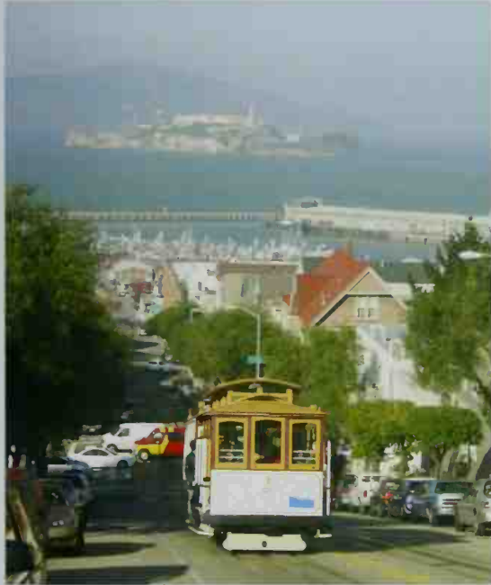
■ In California, San Francisco's famous trolley cars are powered by underground pull cables.
