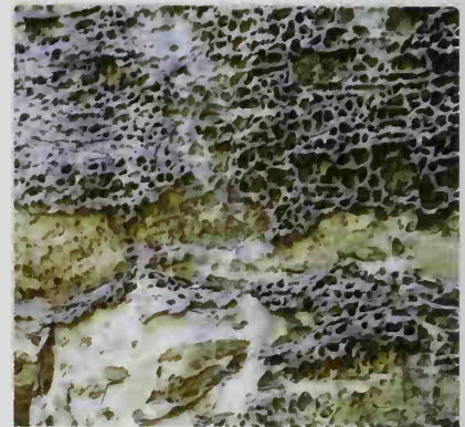
■ Limestone is particularly prone to chemical weathering by carbonic acid in water.
