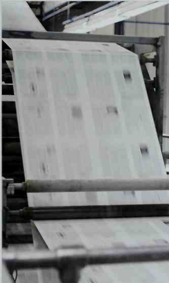
■ Newspapers are printed in large, continuous rolls of paper using offset printing machines.
