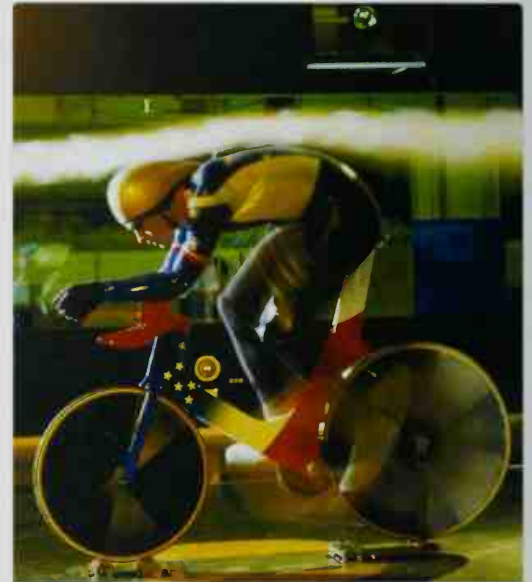
■ Studying the effect of airflow on a cyclist in a wind tunnel.
