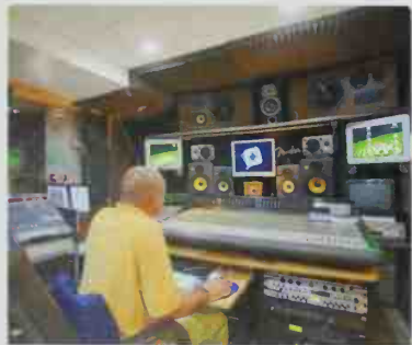
■ At the mixing console, recordings can be combined or "mixed" as desired.
