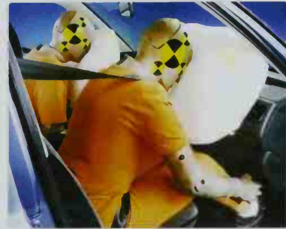
■ In an accident, the head is cushioned from impact by the airbag. Some luxury cars also have side impact airbags in the door.
