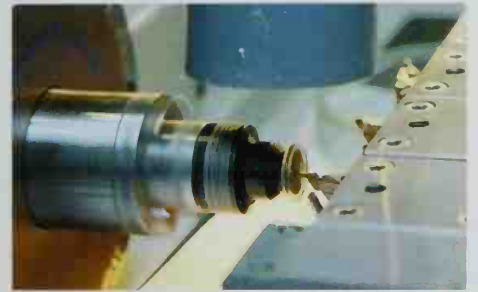
■ Production of a single contact lens with a CNC lathe, a task that requires precision and predictable quality.
