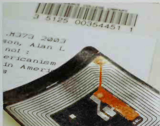
■ RFID tags store information electronically and are replacing more traditional bar codes as product identifiers.
