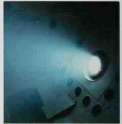
■ The ion thruster engine SMART 1 was used on a probe launched by the European Space Agency (ESA)
