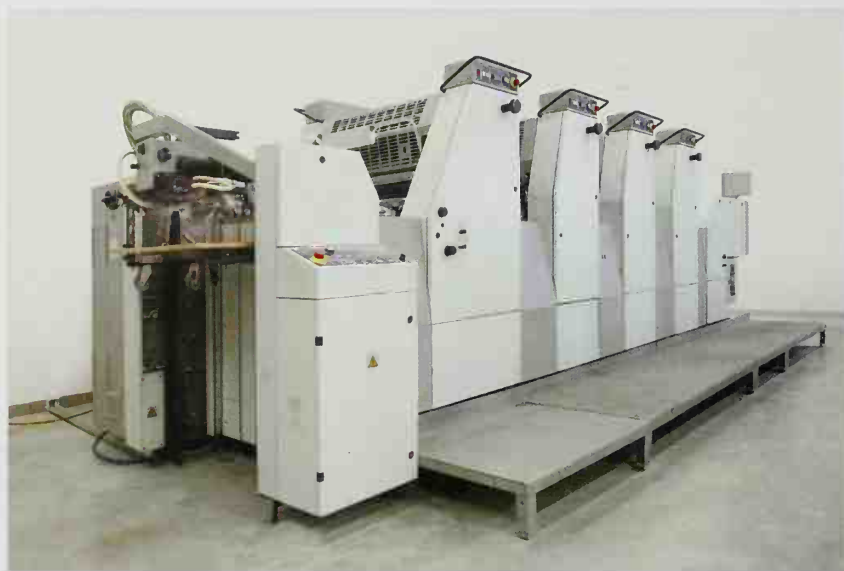
■ Offset printing presses, a development of lithographic printing principles using the interaction of water and oil, are commonly used in commercial mass printing, such as books.
