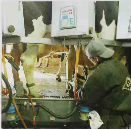
■ Today animals are milked almost exclusively with milking machines. Some milking machines are permanently installed (so-called "milking parlors") and others are mobile for use in tie stalls or in pastures.
