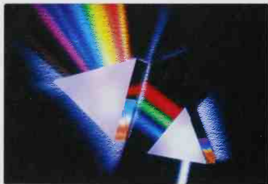
■ A prism splits a white light beam into its constituent spectral colors.
