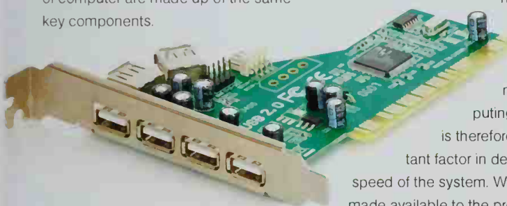
■ A PC expansion board with capacitors, microprocessor, and USB connection ports.
