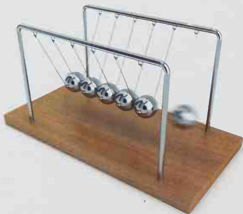
■ Newton's cradle: a device that operates using the principle of the conservation of momentum.
