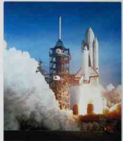
■ The space shuttle accelerates in eight minutes from a stand to an orbital speed of about 17,398 mph.
