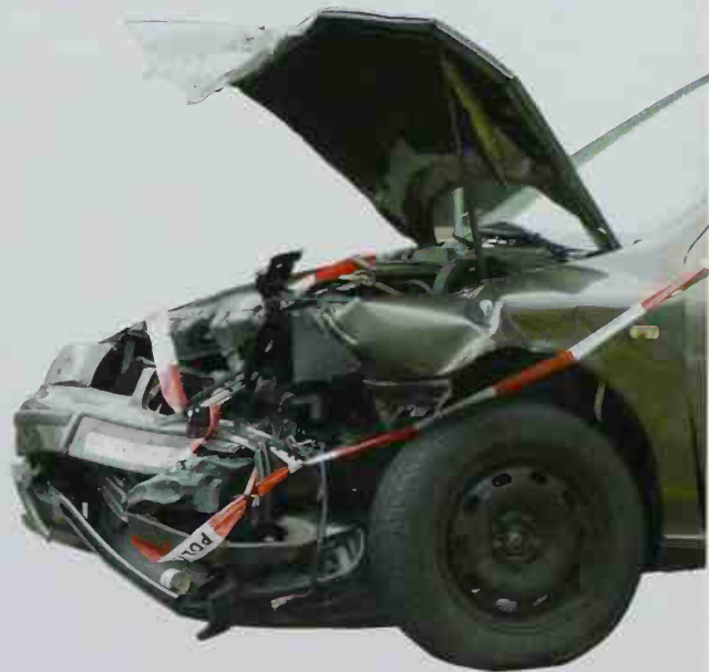
■ The crunch zone effectively lengthens the braking distance. The impact of the collision is thereby lessened.
