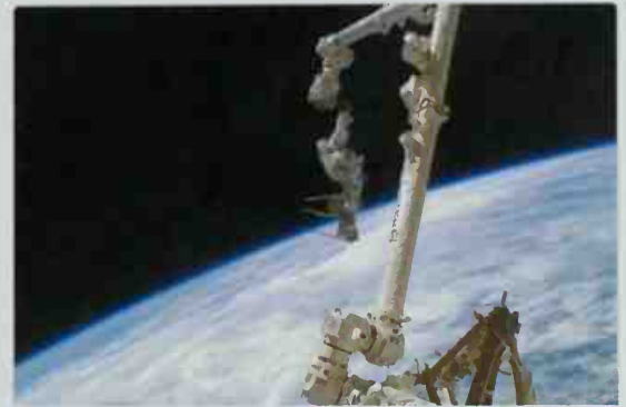
■ The Canadarm is a robotic arm used on NASA space shuttles for maneuvering large payloads in orbit.
