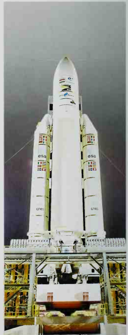
■ Solid fuel rocket boosters are used in staging. They detach from the launch vehicle once their propellant has been used up.
