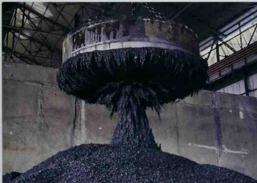
■ An electromagnet can lift many tons of steel scrap metal, vehicles, and cargo containers.
