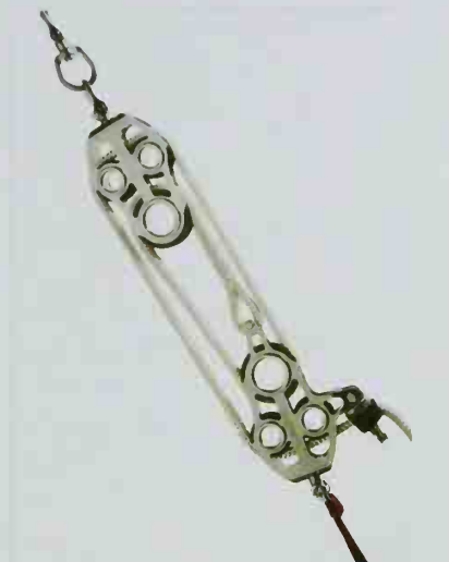
■ A pulley block reduces the force required to pull an object, but the energy required remains the same.
