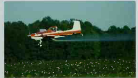
■ Pest control from the air: Crop dusters specially approved for agricultural use have huge chemical tanks and application equipment.
