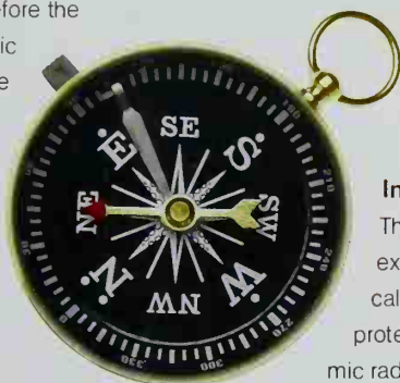
■ A magnetically charged compass needle aligns itself with the Earth's magnetic field.
