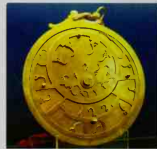
■ The curved spikes on this 18th-century Persian astrolabe mark the brightest stars.
