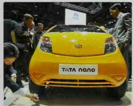
■ Built by Indian carmaker Tata Motors, the four-door Tata Nano, introduced at the New Delhi Auto Show in January 2008, features a two-cylinder engine mounted in the rear of the car.
