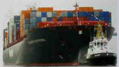
■ The Colombo Express, the world's largest container ship, can load up to 8,750 containers.
