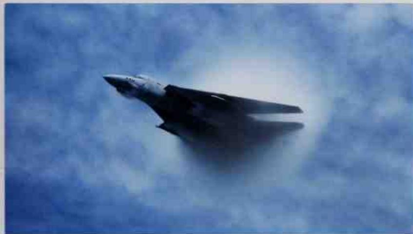
■ During supersonic flight, jet aircraft create pressure waves both in front and behind. The sonic boom is created when the highly compressed forward wave suddenly increases in pressure then is equalized by the rear.
