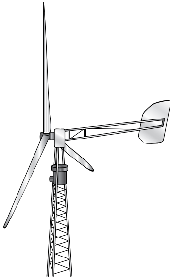
Figure 13-3: Horizontal- and vertical- axis wind generators.
