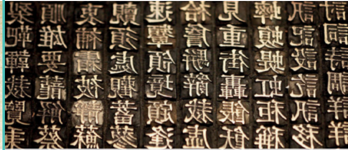
Between 1041 and 1048, Bi Sheng invented the first moveable type printing system, using clay letters held in wax within an iron frame.
